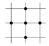
Simple model problem: Jacobi iteration to solve discretisation of Laplace equation
