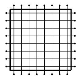
Each block of threads processes one of these grid blocks, reading in old values and computing new values
