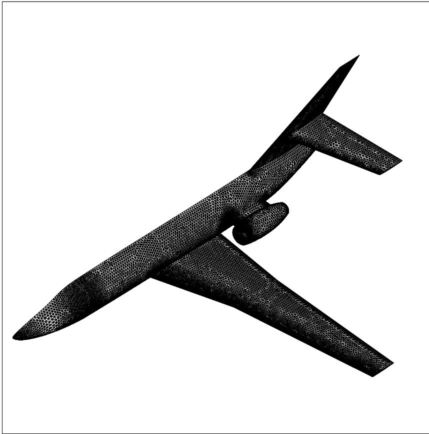
Figure 5: Initial surface grid for aircraft wing design [12]
